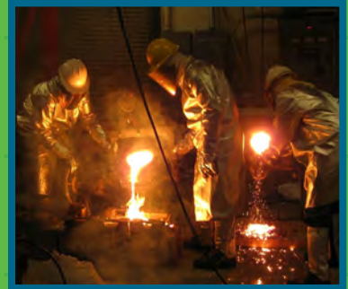
Experimental Pour of Gen3 Lightweight Steel
